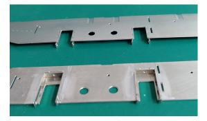
upside down. The kit is deigned to be fitted with a ABC Mini S and a mounting \_\_\_\_\_ bracket (7) is incorporated as part of the spacers, (4) is at front and spacer (8) at the rear of the chassis. There is a "F" for front etched on the inside front of each frame. Dry fit all the five parts to ensure they all slot together, when satisfied with the fit, with the chassis upside down on a flat surface, tack solder together.
