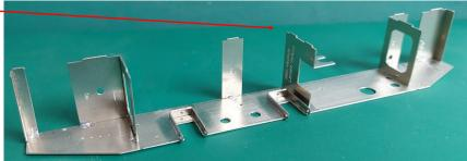
14. Check that all is flat and square and the solder fully. Rub down the outside of the frame so that no tabs protrude.
