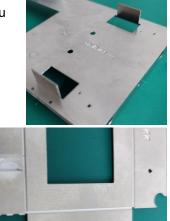
32) Now to the "origami" bit. Start by folding the "top" at 90°, next fold the outer side to 90° and then make the last long fold "base" at 90°, lastly fold in the tank front. Tweak until you have a nice square box and when satisfied solder the long and end seams. Repeat for the other tank. Finish by soldering a piece of tube into the circular pockets around which the overlay will roll.
