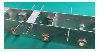
with a fine square needle file. At all costs avoid a sloppy fit. Now fit the crankpins as per instructions that came with the wheels. There are some etched washers on Sheets 98 & 99 if you want to reduce the side play in the wheels.
